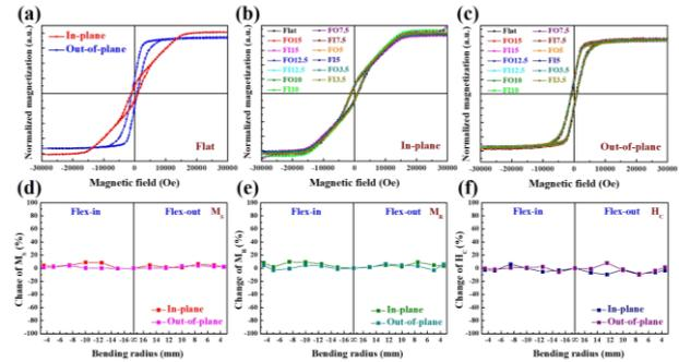
Fig. 4 Hysteresis loops under various bending radius
