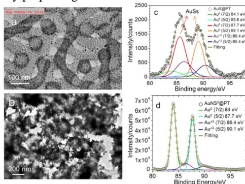
Fig. 2. (a-b) TEM images and (c-d) XPS Au<sub>4f</sub> spectrum of AuSs@PT (a,c) and AuNSs<sup>3</sup>@PT (b,d), respectively.
