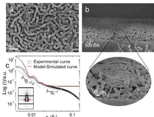
Fig. 1. Structural characterization of a PT sample obtained through SR in hot EG at 130 °C (15 min). (a) Top-view and (b) side-view SEM images. (c) GISAXS 1D in-plane profile. The inset of Figure 1b is a zoom-in image and the inset of Figure 1c is a 2D GISAXS pattern.
