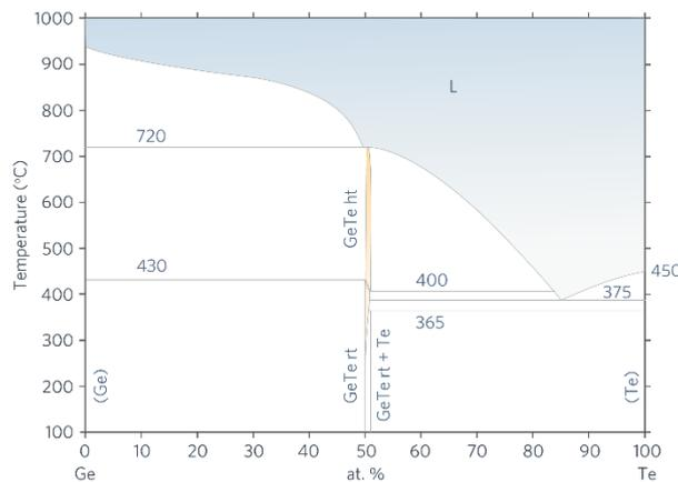
**Fig. 1** Ge-Te binary phase diagram [3].
