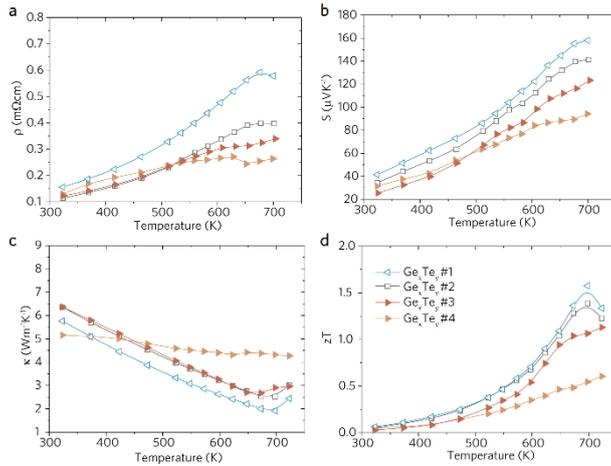
**Fig. 3** Temperature-dependent (a)  $\rho$  electrical resistivity (b)  $S$  Seebeck coefficient (c)  $\kappa$  thermal conductivity (d)  $zT$  value of GeTe through compositional control.
