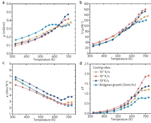
**Fig. 2** Temperature-dependent (a)  $\rho$  electrical resistivity (b)  $S$  Seebeck coefficient (c)  $\kappa$  thermal conductivity (d)  $zT$  value of GeTe through controlled cooling rates.
