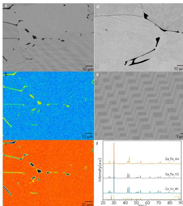
**Fig. 4** The metallographic observation of  $\text{Ge}_x\text{Te}_y$  alloys (a) backscattered electron image (BEI) of  $\text{Ge}_x\text{Te}_y$  #2, elemental mapping results from (a) of (b) Ge and (c) Te, (d) backscattered electron image (BEI) of  $\text{Ge}_x\text{Te}_y$  #1 (e) Magnify the BEI from (d), (f) XRD patterns of  $\text{Ge}_x\text{Te}_y$  alloys.
