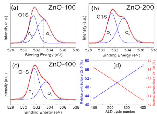
**Fig. 1.** (a)-(c) O1s XPS bands of ZnO thin films. (d) Linear dependency of presence of Zn-O and Zn-OH bonds in ZnO thin film from cycle number of ALD.
