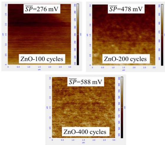
**Fig. 2.** Surface potential mappings of ZnO thin films.
